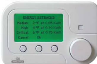
Displays energy rates allowing money savings on energy bills if rates change.*
