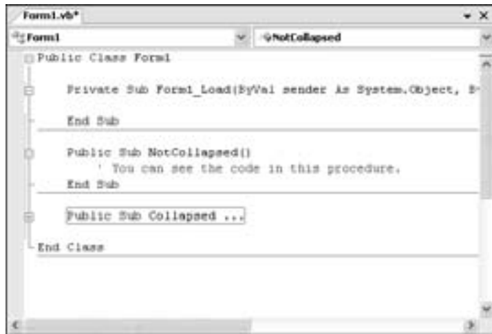
Figure 2-11: Collapsible code without a region
